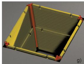
f) If the plate head has reached the upper edge of the pit, insert a second plate into the inner guide of the corner slide rail if necessary, as far as the height of the blade of the first plate. Press in the inner plate further, as described in e) If necessary, slide support plates to the outer slide-rail guide and connect them to the lower plate by means of locking bolts and safety clips.
